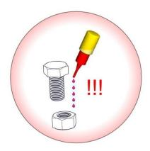
Glue all screws, nuts and sleeves with loctite. (not less than 5 drops!) (except for Nylock nuts)
