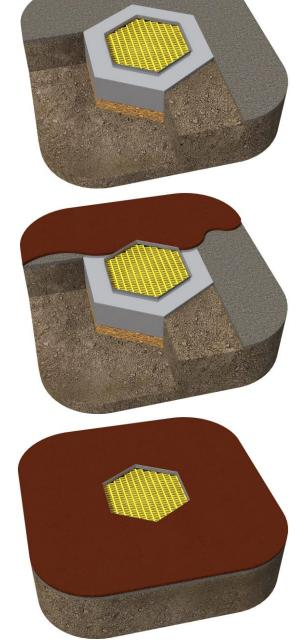
**Step 4**Unscrewing and removing the formwork strip
