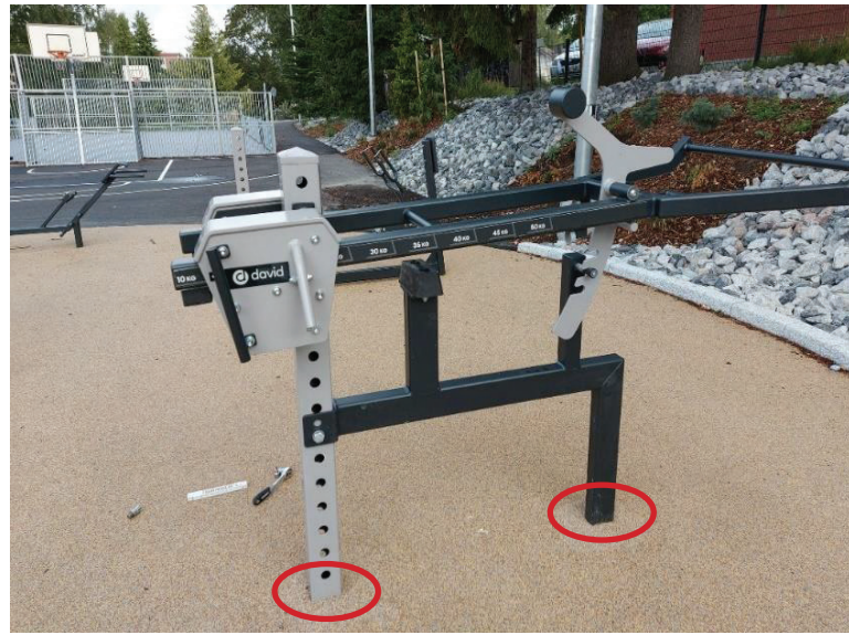
Device mounted on a soft safety platform Mounting Post and the fixing bolts must remain visible
